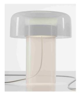
Tech. description The light comprises a glass shade surrounding a metal cylinder with a 24V LED module fitted on each side and a power cable with dimmer box, which houses the power source (LED driver), dimmer, and power switch. The dimmer allows adjustment of the brightness of the LED module and the direction of the light (up only, up and down, down only).
